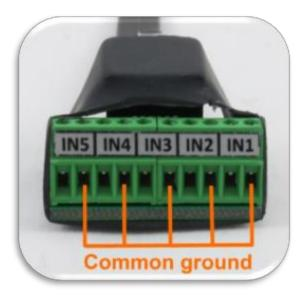
Up to five external switches can be connected to LX Eos. To connect external switch to LX Eos you have to use external switch interface board (included in package). Every slot available has a signal input and ground input. The configuration of inputs can be set under Setup -> Inputs.
