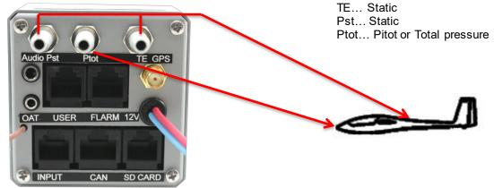
TE tube installation schematics (Set TE 0%)
